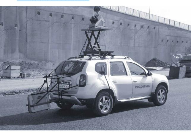
Carrying out special inspections of transport infrastructure facilities to establish causes of deformation of road (airfield) structures and disruptions of roadbed stability, substantiate design solutions within the framework of major repairs and reconstruction, as well as control quality and volume of road construction work performed. Preparation of proposals for the elimination and further prevention of deformations and destruction.
